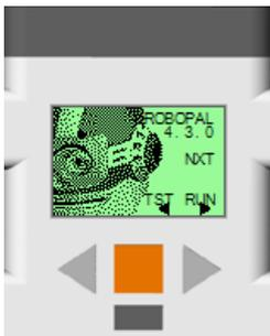
RoboPAL transmits the program to the NXT via a Bluetooth connection. A special RoboPAL dongle is required for this. The program that runs on the NXT is a very compact version of the program that runs on the PC. This makes transmitting the program fast. The NXT needs to be switched on and the firmware needs to be running. When starting the NXT, the default LeJos firmware will start, followed by the RoboPAL start-up screen (as shown in the picture).
