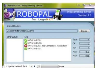
The server first needs to find all NXT units (just as on the PC) by using <refresh local list>. After the robots have been identified, a list is created on the server called BRICS.TXT. This list is retrieved by all the PCs that use the server, by selecting <refresh network list> in RoboPAL on the PC. This will retrieve the server list and creates a list on the PC of all NXT units that can be used through the server. You will need
