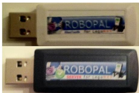
The special RoboPAL dongle takes care of all actions such as registering and connecting to Bluetooth. In addition, the dongle also serves as a software license for the RoboPAL software. Without a dongle, programs will not upload to the NXT. This dongle is ONLY usable with RoboPAL and cannot be used for other Bluetooth devices.
