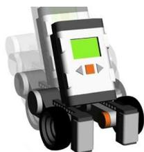
Using a simpler programming language and a standard Lego NXT robot not only makes programming simpler, but also allows the robot to be used for other projects. The Lego NXT is a flexible robotics construction set that can be programmed with a large range of programming languages. Moreover, a large variety of sensors and other equipment is available. This makes it possible for students, after following the RLT robotics course, to work on larger projects independently.
