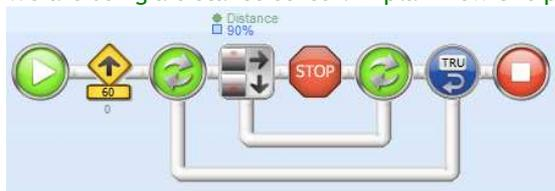
*The robot drives forward slowly. If the distance sensor detects a value higher than 90%, the robot will stop.*
