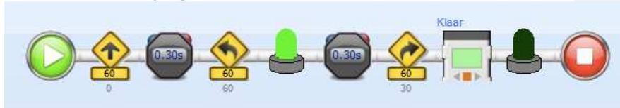
*It makes the robot drive forward 0.3 seconds, make a left turn for 0.3 seconds and then turn on the green lamp. Subsequently, it makes a left turn for 1 second (default), displays "Ready" on the LCD screen, turns off the green lamp and stops.*
