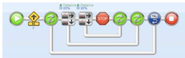
This code checks whether a value is higher than 60% and lower than 90%. It is used to see if a value is between two limits.
