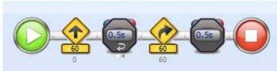
The first icon with a stopwatch is a LoopTimer that needs a wire running back to the beginning of the program, but the line is missing.
