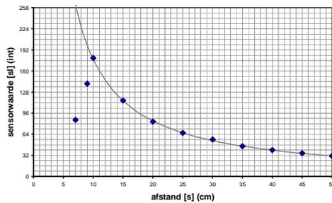
According to the graph, the value at 15 cm is about 120. Although the graph shows a maximum value of 250, the standard maximum is 1023. So:  $120 / 1023 * 100 = 12\%$
