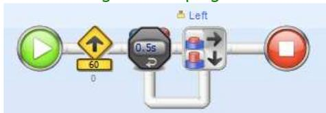
The output of the sensor test is connected to the output of the stopwatch, but it should be connected to an action later in the program, which is missing. The construction shown here has no sense, so the program will ignore the sensor test.
