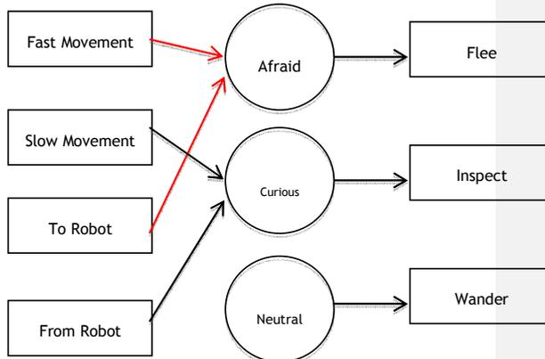
In these programs, it is important to make use of a State Diagram, which defines the states that a robot can adopt along with their associated actions. This is a further refinement of the Sense-Reason-Act loop.
