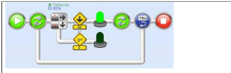
In this program, turning off the green LED is not connected with the Merge icon above it.
